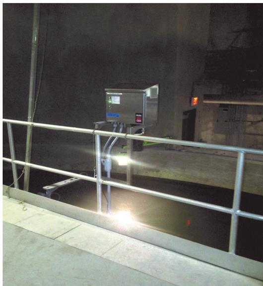
Portable instrument to measure sludge blanket level in clarifiers and thickeners. Blanket Tracker is a portable optical meter for measuring of sludge blanket depth and suspended solids in clarifiers, thickeners, aeration basins etc in water and wastewater plants, as well in other facilities.
