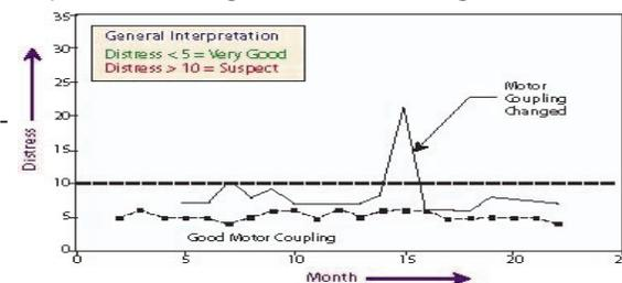
1. instantly alert to the presence of a fault on a machine without knowledge of machine details (such as bearing type or number),
